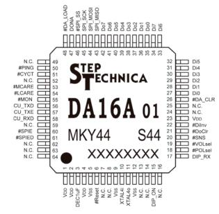
$Note: N.\ C.\ pin is\ not\ connected.\ Pins\ prefixed\ with\ "\#"\ are\ negative\ logic\ (active\ Low).$
