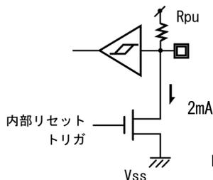
$V_{t+} \text{ max} = 2.1\text{V}$
